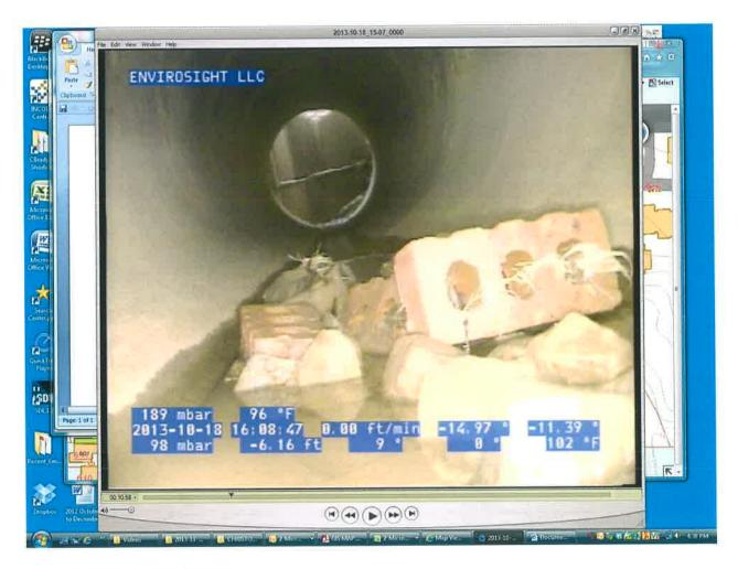
Photo 1: debris in pipe, 24" RCP,
