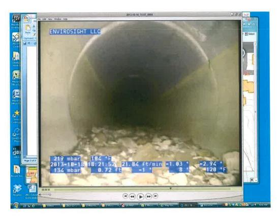
Photo 4: debris in pipe, 24" RCP
