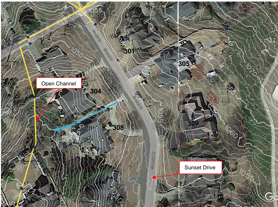
Figure 3 – Natural Direction of Flow from the Golf Course. Google Earth Imagery dated March 2022.
