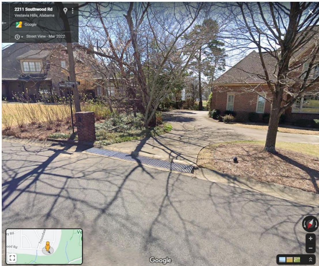
Figure 9 – The typical grated driveway spanner that is recommended is located at the property of 2211 Southwood Road. Google Imagery dated March 2022.
